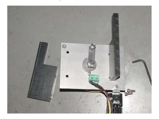
When we install the Institute in the side tracks, we will need to align the cam with the institute track. This picture does not show how it is mounted, it just shows where the cam mounts.
