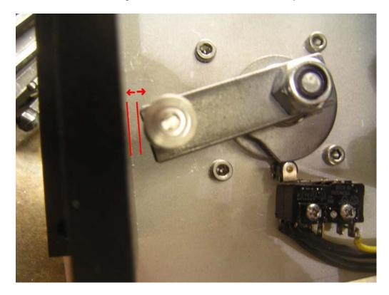
The switch is adjusted with the screws shown below. You should not have to adjust this as they were properlyadjusted prior to shipment. The screw circled in blue is a pivot point and the actual adjustment is made using the switch on the left (circled in red). You may need to loosen the nut on the back of the unit to properly adjust the switch.
