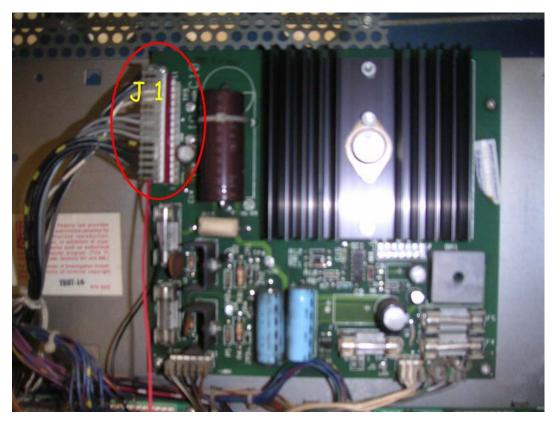
When complete, feed the wires through the backbox to the under side of the playfield. We are now going to test the unit. Connect the other end of the wiring harness to the motor unit.
