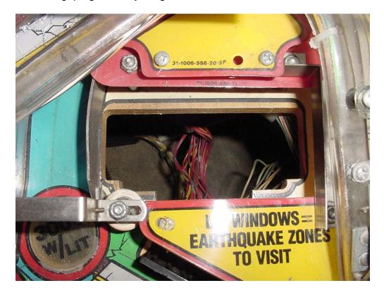
Move the institute to a clean static free place. Locate the two screws that hold the lamp PCB to the institute's plastic frame. Remove these screws with a Philips screw driver.
