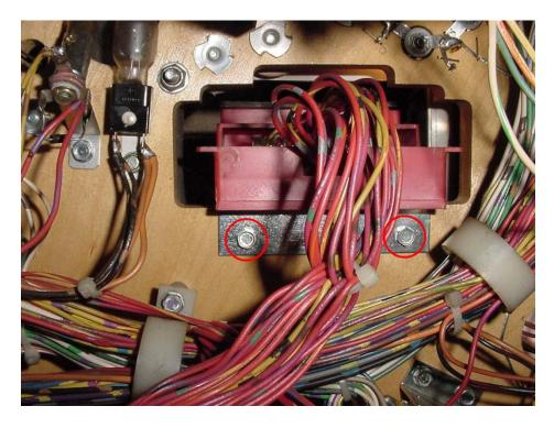
Carefully remove the wire connector from the bottom of the institute. Use a ¼" nutdriver or a small ratchet to remove the screws.Retain the screws to later install the motor unit.
