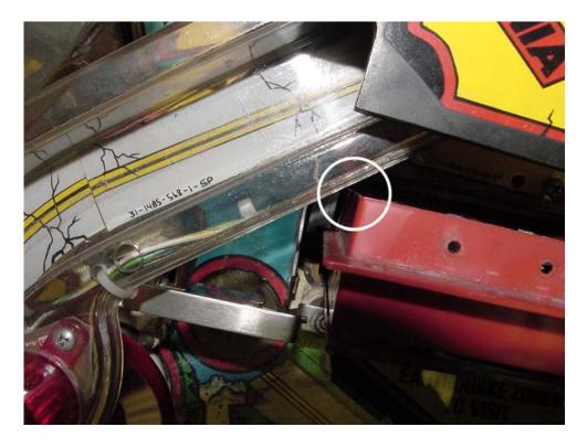
Use the two screws we removed that held the institute in originally, backed with the two washers we supplied, to secure the institute to the playfield. You will need push hard when inserting the screws so that they tap new holes in the underside of the playfield. You can drill pilot holes to make the process easier, but there is a danger of drilling through the playfield or catching some wires with the drillso we're leaving this to your discretion.
