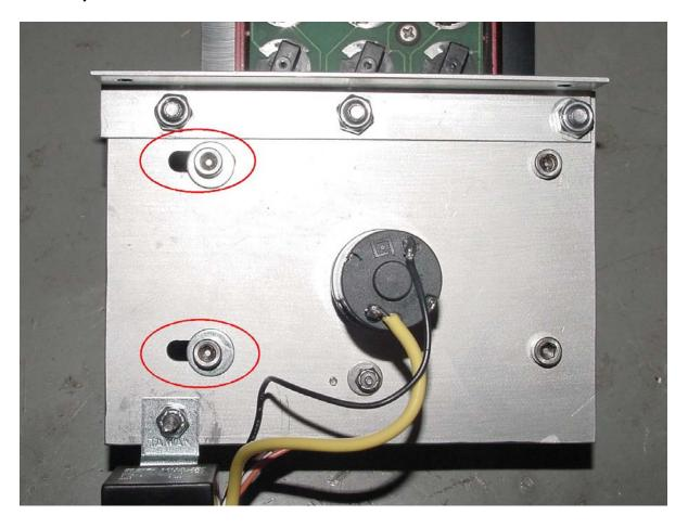
Be careful when adjusting the rails not to get too close to the Cam Follower. Contact between the cam followerand the risers will damage the unit so be careful not to adjust the riser too close.
