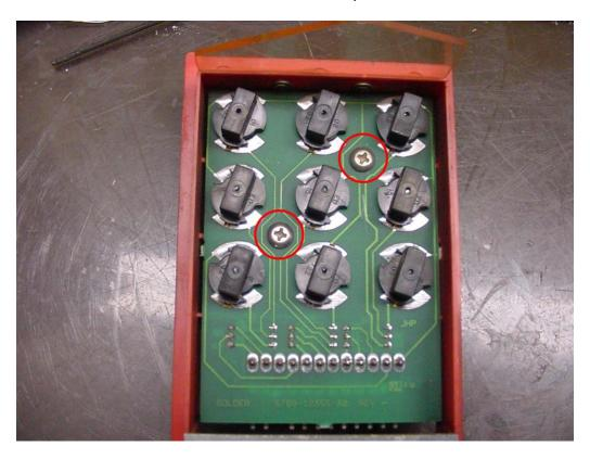
We are now going to have to remove the two rivets shown belowto remove the mounting bracket.
